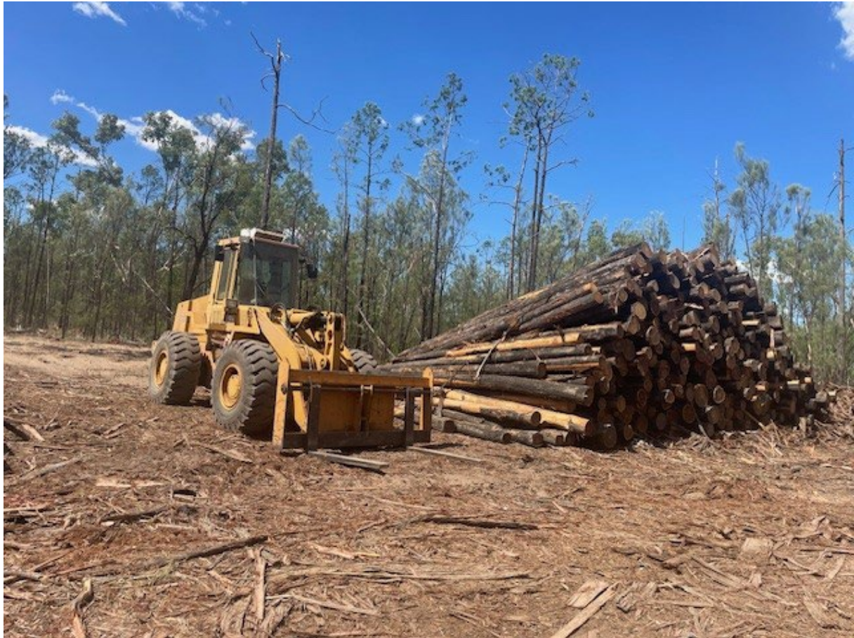
Figure 5 – Loader without log grab being used to load Cypress logs.
