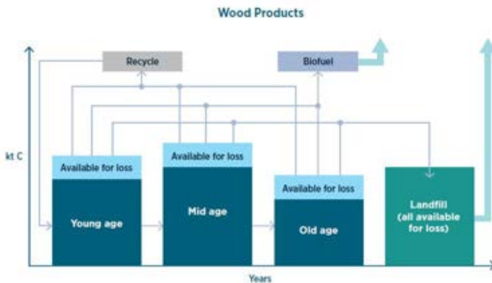
Figure 3.9. Illustration of the National Wood Products Model depicting the annual proportion of products lost from each age class and designation of end-of-life streams (Australian Government, 2023a)
