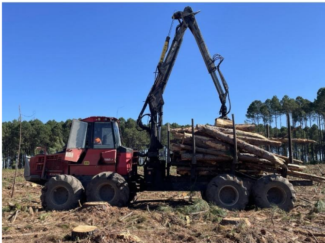
Forwarder recovery of harvest residues following cut-to-length at stump harvest operation (14 Landsborough, higher residue levels than usual on this ex-CSIRO pasture research site)
